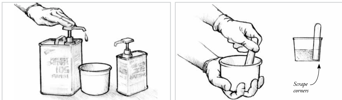
Figure 16-4 Dispense the proper proportions of resin and hardener. Figure 16-5 Stir resin and hardener together thoroughly, at least one minute—longer in cooler temperatures.
