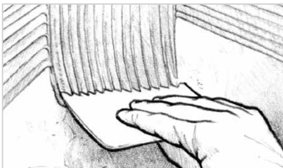
Figure 14-7 Apply the fairing compound with the notched spreader. Control the height of the ridges by the angle you hold the spreader.
