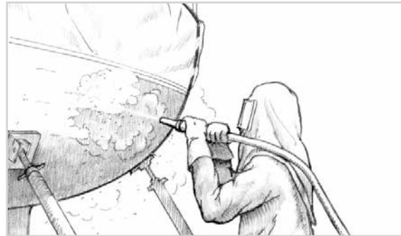
Figure 10-3 Sandblasting is a common method of opening blisters and abrading the hull.
