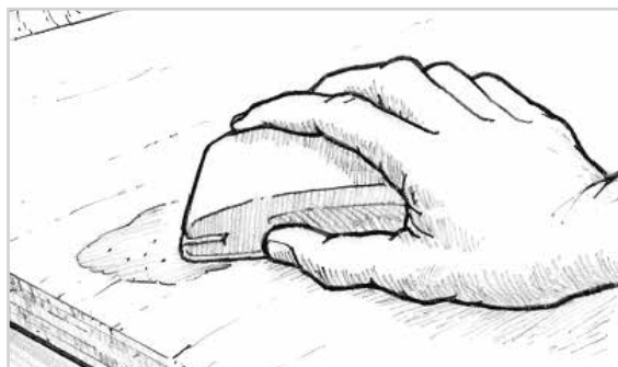
Figure 16-16 Sand the fairing material to blend with the surrounding contour.
