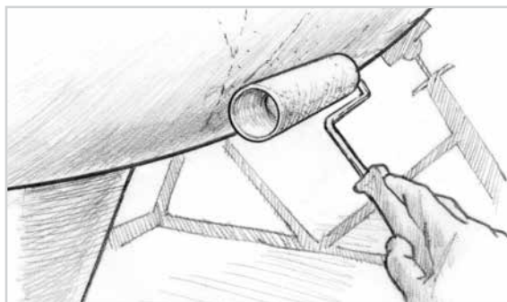
Figure 1 Apply a coat of unthickened epoxy to the hull.
